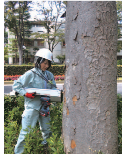
Diagnosis using resistograph
